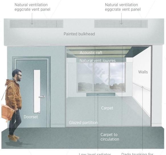
Low level radiator providing perimeter heating Dado trunking for power & data points - 870mm from floor level
