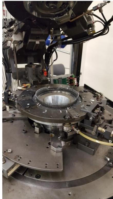
Figure 5 Close up of circular knit needle bed
