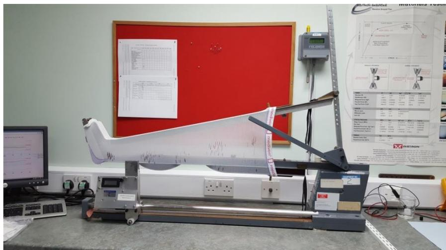
**Figure 1 Hatra Mark II - Graduated compression garment test equipment utilised as part of the British Standard.**
