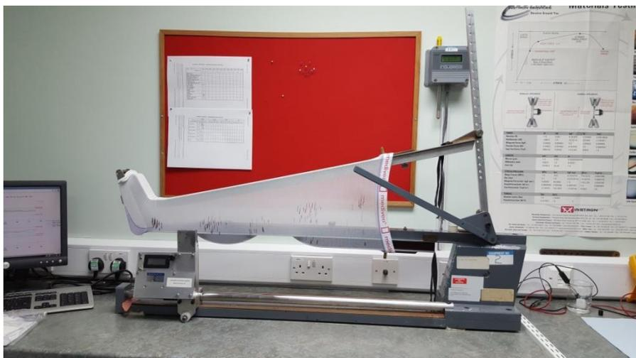
**Figure 1 Hatra Mark II - Graduated compression garment test equipment utilised as part of the British Standard.**
