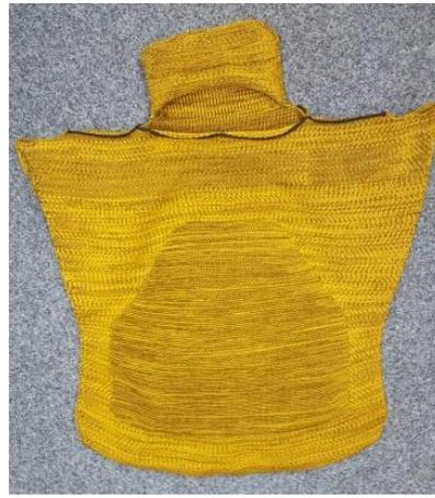
**Figure 13** Camira knitted pattern piece before being fitted onto chair frame.
