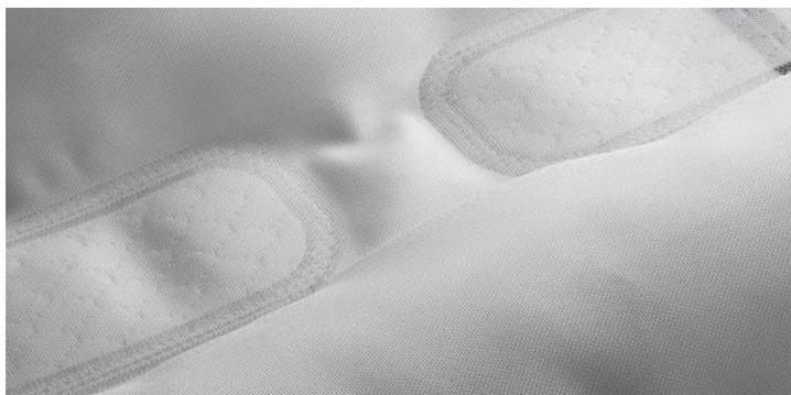
Figure 17 Close up detail of woven airbag [2]
