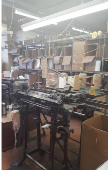
**Figure 10 Manual double bed knitting machine utilised at Sallis Healthcare**
