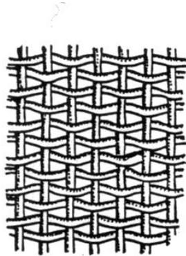
Figure 15 Illustration of woven fabric
