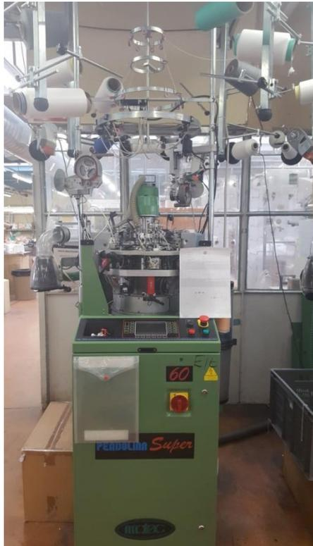
Figure 4 Circular knitting machine utilised at Sallis Healthcare
