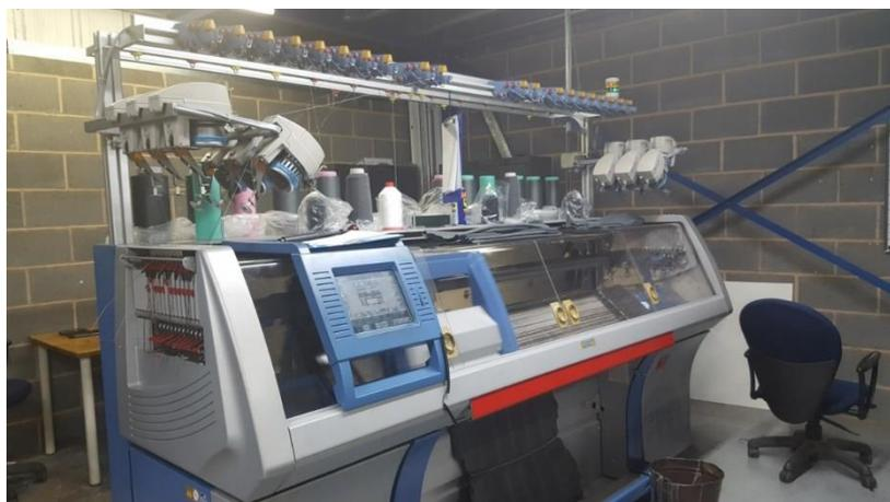
**Figure 11 Stoll multi gauge knitting machine utilised at Camira Technical Knit**
