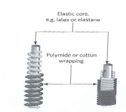
Figure 14 Illustration of two-core spun yarn [1]
