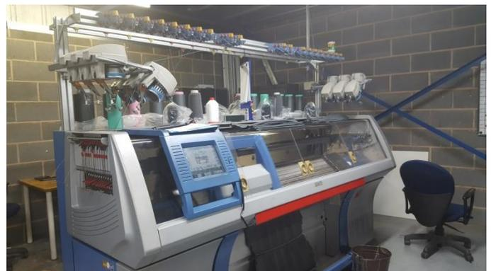
Figure 8 Stoll multi gauge knitting machine, Camira Technical Knit
