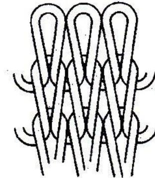
Figure 16 Illustration of knit fabric
