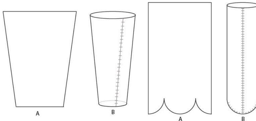
Figure 6 Illustrative examples of simple flatbed designs where drawings marked (A) represent the knitted pattern pieces and drawings marked (B) represent the stitched garments
