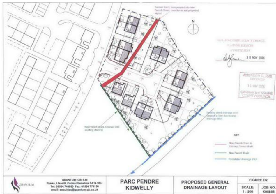
Figure 15 – Map of the approved surface water drainage design for Clos Yr Helyg (Quantum, 2006).
