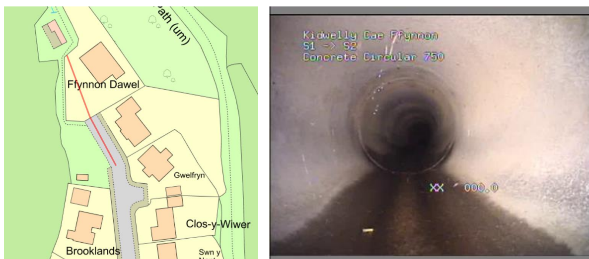
Figure 28 - The private section of culverted watercourse at Cae Ffynnon Kidwelly.
