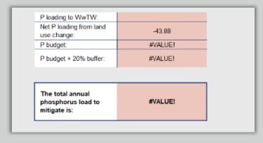
This value shown in the Net P loading from land use change cell demonstrates that the mitigation scheme will remove 43.88 kg TP/year. This suggests that the mitigation scheme will provide additional nutrient mitigation than what is needed for the site. However, it is likely that further information would be required to demonstrate the timescales of the land use change and the nutrient reduction to the site.
