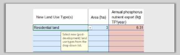
In this example, the developer has also provided evidence to demonstrate that onsite SuDS features will be used in a treatment train approach and will drain all of the surface runoff from the site. The developer has also provided information to show the SuDS will be able to remove 40% of the TP in the surface runoff.
